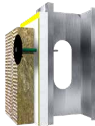
Continuous exterior insulation attached over air & water barrier with gasketing tube seal fasteners.
