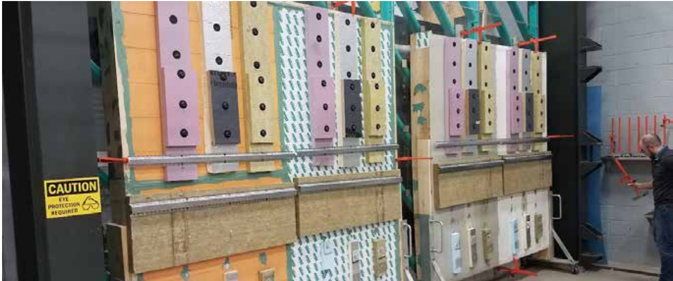
Water and air test wall assemblies with various air barriers and overlaying insulations penetrated by various tube seal fasteners including brick anchors, insulation, lath, and channel attachment.
