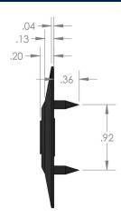
Basis of Design: Thermal-Grip® ci Prong Washers as manufactured by TRUFAST Walls.
