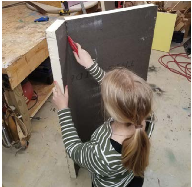
Cutting the roof panels to cap the mini "hot box". Almost ready for testing.
