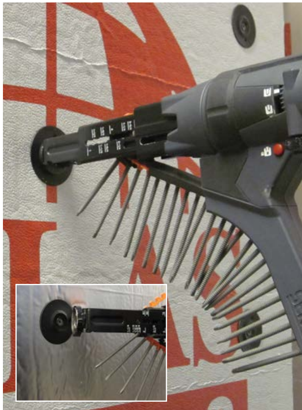
Auto-feed screw guns with custom washer adaptors are significantly faster than bulk screws and washers. Invest in the right tools for the job to cut costs without cutting corners.
